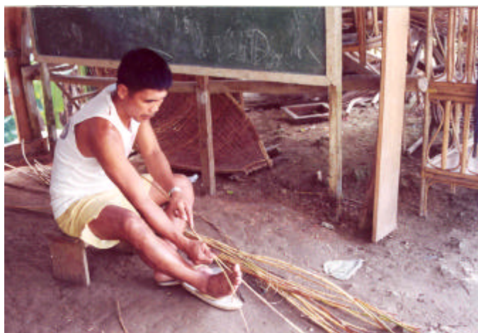
Practice of rattan splitting
