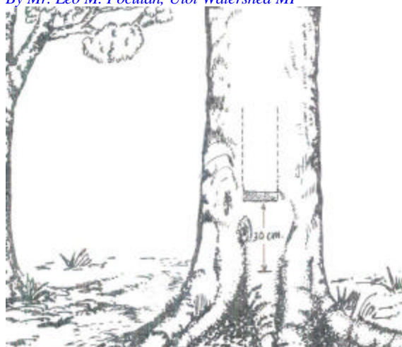
Fig.2 Start first cut not more than 30 cm from the ground or above buttress
